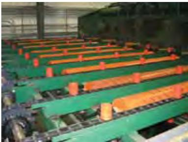
**Redco™ Diverter Arms** are impact resistant, with a low coefficient of friction. Their lightweight construction allows the arm to tip up and down quickly with low inertia.
