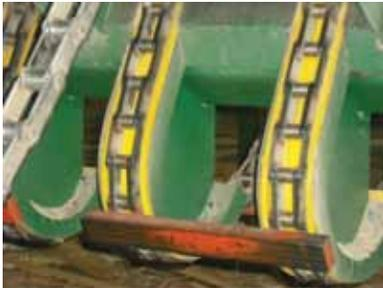
**Redco™ Snap It Sprockets** are installed easily - simply snap into place. Redco™ Sprockets are much less expensive than split steel sprockets and reduce maintenance downtime, therefore increasing production.
