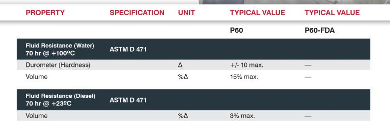
Unless otherwise stated, all Redco sheet rubber is provided to standard RMA Rubber Tolerances.
