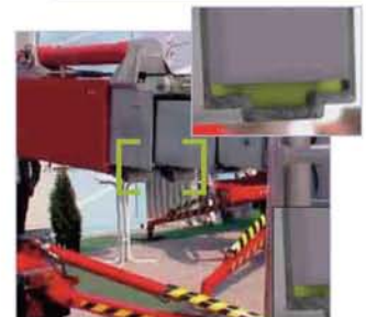
TIVAR® Ceram P® performs well as a slide panel in telescoping booms. Outstanding abrasion resistance adds to the wear-life of the pad.
