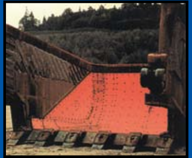
Dragline Bucket Liner
